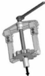
Continue pulling until the part to be pulled is completely loose.
