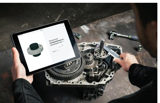
**2.** Then the specific data such as the inner or outer diameter, size of the clamping depth as well as the space next to the part to be removed must be entered. Each individual input from the user affects the product search. This always guarantees that the extraction tool required for non-destructive dismantling is also found.
